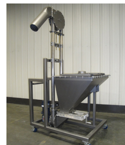
Mobile aero mechanical conveyor & hopper
