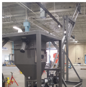
Mobile bulk bag unloader with flexible screw conveyor & aero mechanical conveyor with hopper
