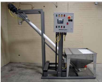
Mobile flexible screw conveyor, hopper & control panel
