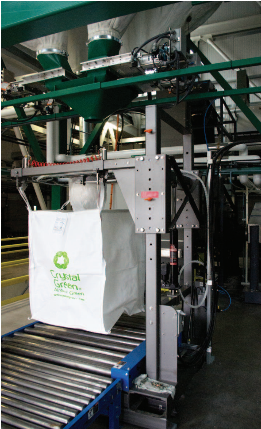
After a bulk bag is filled, the bag-filling system's powered roller conveyor moves it out of the filling zone to an indexing roller conveyor.
