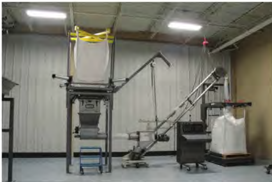
The supplier's test lab equipment shown here includes a bulk bag discharger, flexible screw conveyor, aeromechanical conveyor, and bulk bag filler.
