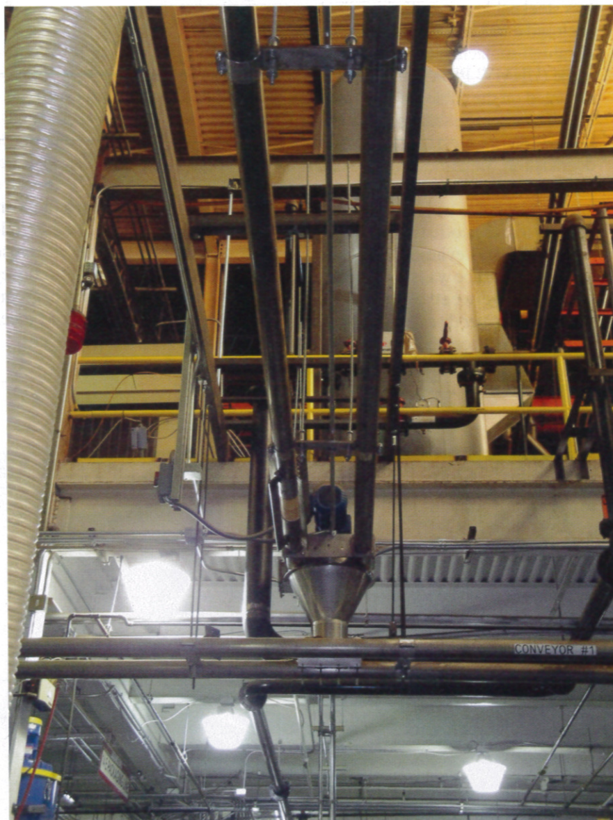
The roasted beans discharge from holding silos into a tubular drag conveying system that moves them vertically and then horizontally above the plant's coffee grinders.
