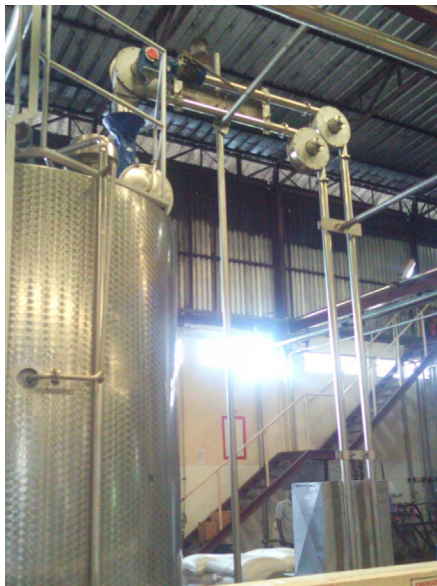
Aero Mechanical Conveyor in the brewery
