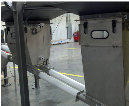
Bulk Bag Unloading System with dual Flexible Screw Conveyors
