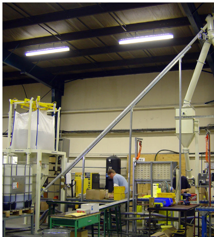
The flexible screw conveyor transfers silica sand 18ft/ 5.5m high over a distance of 16ft/ 5m.
