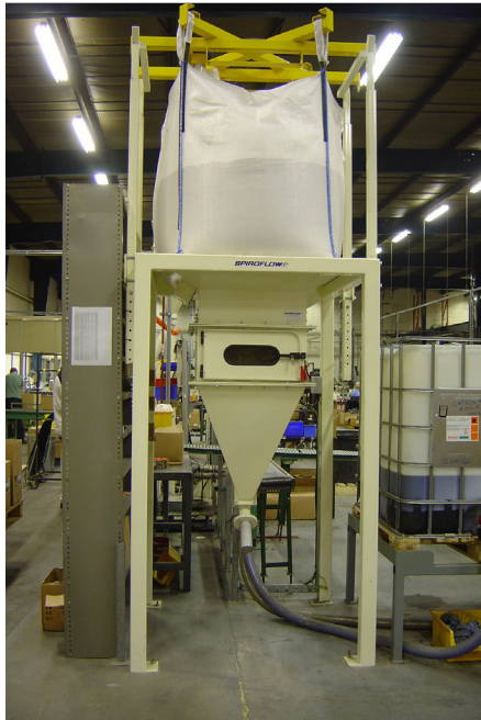
The bulk bag unloader supplied to unload silica sand.
