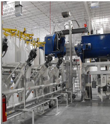
Rear of the Unloaders showing the Flexible Screw Conveyors feeding the Aero Mechanical Conveyors
