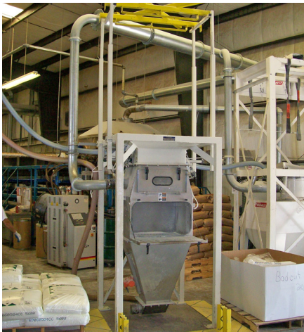
Bulk Bag Unloader with spring-loaded arms
