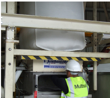
Operator Untying a Bulk Bag
