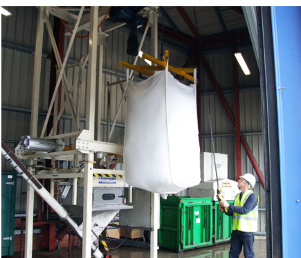
Bulk Bag being hoisted into the Spiroflow Bulk Bag Unloader
