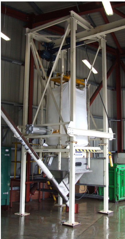
Spiroflow Bulk Bag Unloader with Flexible Screw Conveyor Leading Off to the Left
