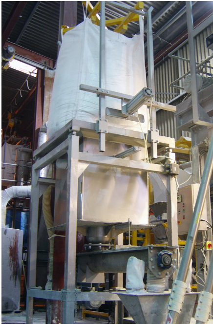
Bulk Bag Unloader handles moisture-sensitive chemicals
