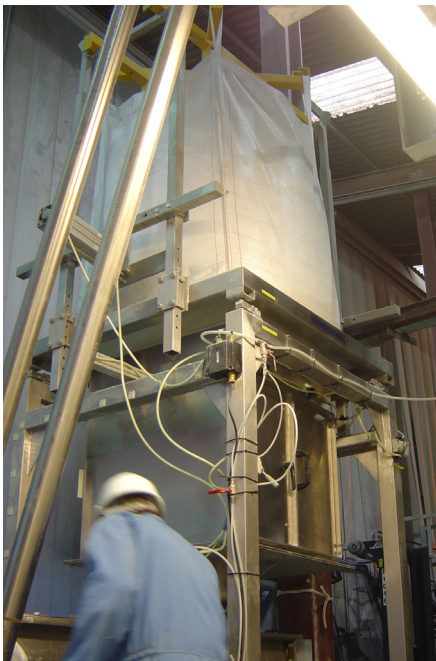
Bulk Bag Unloader handles moisture-sensitive chemicals
