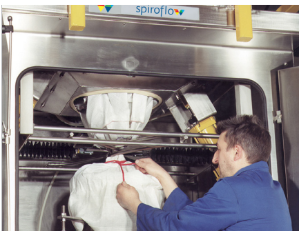
Pinch bars keep the neck of the bag closed while it is untied.
