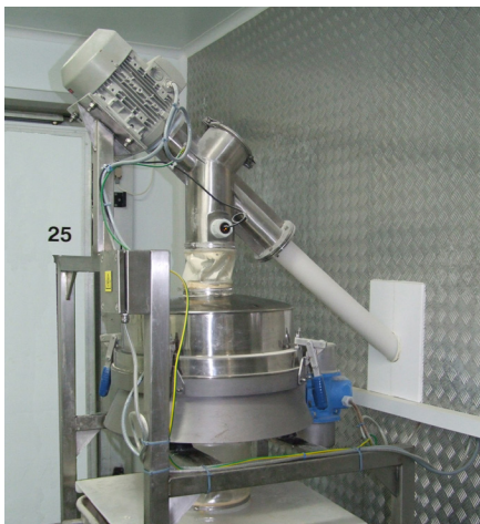
Outlet of Flexible Screw Conveyor unloading bread crumbs via a sifter in to tubs
