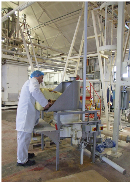
Operative charging sacks of brown flour directly into the mixer via the additional conveyor
