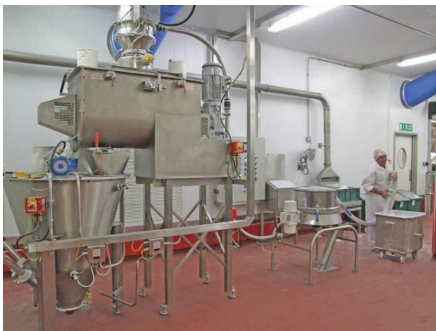
The suction wand transfer system to the mixer with the buffer hopper below
