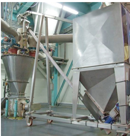
Cocoa powder being conveyed to mixer with Spiroflow's Flexible Screw Conveyor
