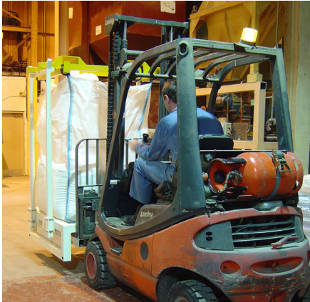
Bulk bag being loaded into top section at floor level
