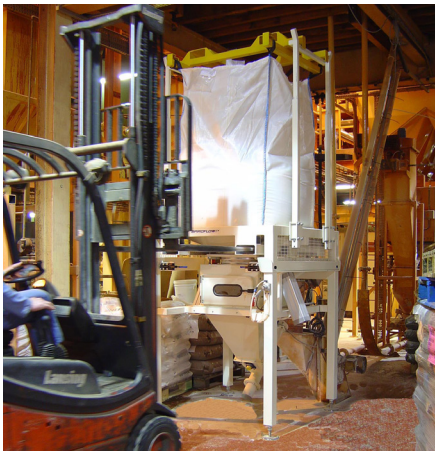
Top section with bulk bag returned to the unloader and lowered onto the base.
