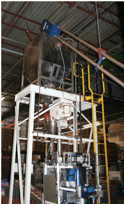
The Aero Mechanical Conveyor delivers coffee blends to the buffer hopper on top of the packaging machine.
