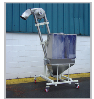
An AMC with a bag dump hopper & integral dust hood.
