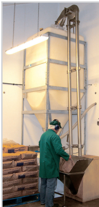
An AMC is used to unload sacks of sugar into a storage hopper.
