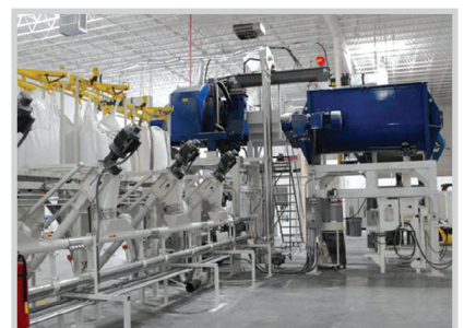
An AMC with multiple inlets delivers cement, sand, ash & recycled glass to a second unit that lifts them up into a mixer.
