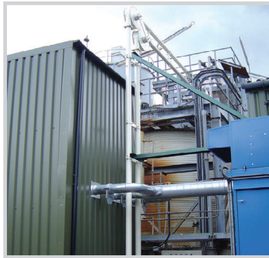
An around the corner Aero Mechanical Conveyor feeds chemicals to a mixing vessel.
