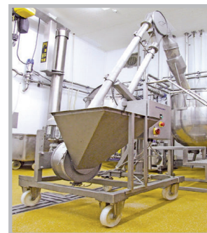
An AMC with a simple bag dump hopper for non-dusty materials.
