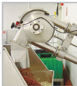
Interlocked inspection hatch in sprocket housing.
