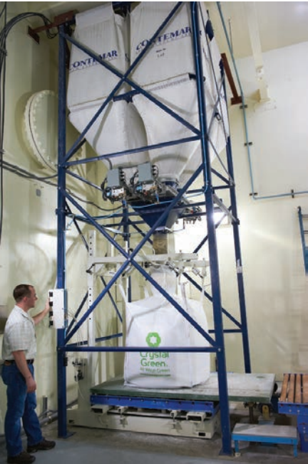
ABOVE: The Durham plant is the first in the nation to successfully employ the Ostara technology. The $2.5 million system produces about 300 tons of Crystal Green fertilizer a year. RIGHT: Operator Brett Laney loads prills for shipment using the Spiro-flow conveyor with Siemens control panel and fabric silo from Contemmar Silo Systems.
