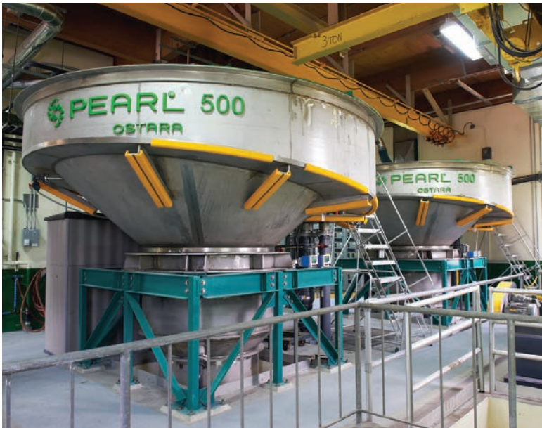
ABOVE: The Durham plant is the first in the nation to successfully employ the Ostara technology. The $2.5 million system produces about 300 tons of Crystal Green fertilizer a year. RIGHT: Operator Brett Laney loads prills for shipment using the Spiro-flow conveyor with Siemens control panel and fabric silo from Contemmar Silo Systems.
