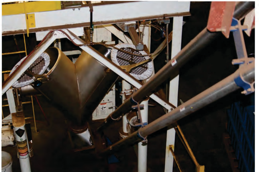
The Model PC3 Aero-Mechanical Conveyor (AMC) from Spiroflow Systems at Excelso Coffee & Tea Company in Norcross, GA is used to convey flavored coffee from a V-Ribbon blender to a storage hopper.
