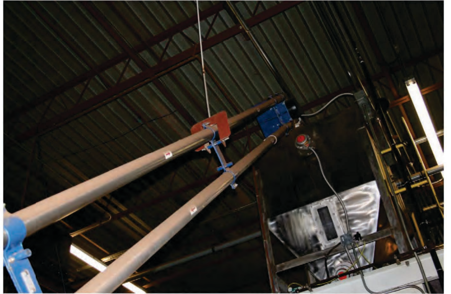
The Model PC3 Aero-Mechanical Conveyor (AMC) feeding the V-ribbon blender.
