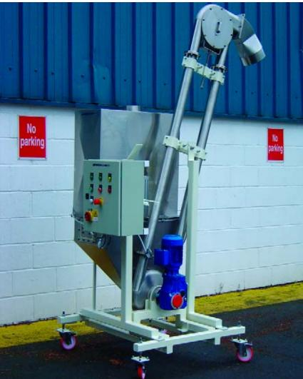
An operator can easily move the mobile aeromechanical conveyor onto a floor scale located near a mixing vessel.
