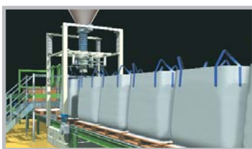
Semi-automated bulk bag filling system.
