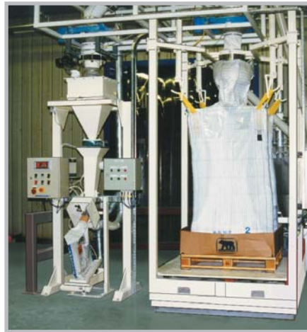
Filling system for bulk bags and 50lb bags.
